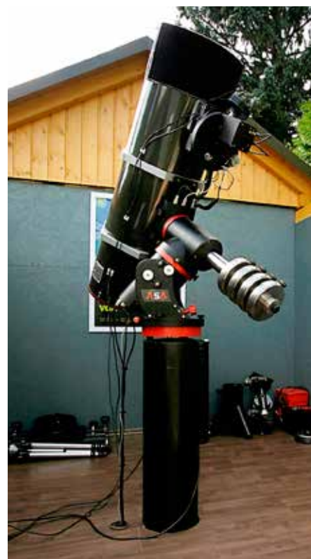
The author's remote-controlled observatory in Eichgraben, Lower Austria, contains a 12-inch ASA 12N astrograph at f/3.6 on an ASA DDM85 mount. He also observes from the Austrian Voralpen and Namibia, where he has a remote setup.
